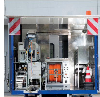
Expansion of a sewer inspection truck with high-pressure flushing unit
