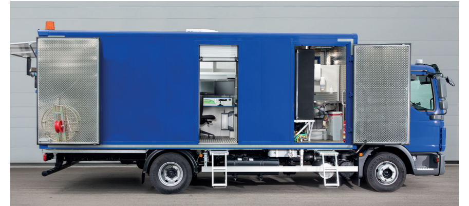
Expansion of a sewer inspection truck with high-pressure flushing unit
